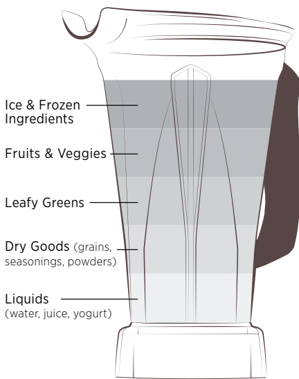
Loading the Container
