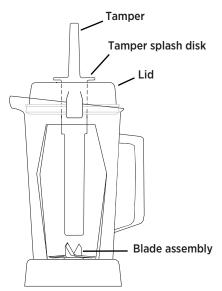
Holding the tamper straight down may not help the ingredients circulate.
